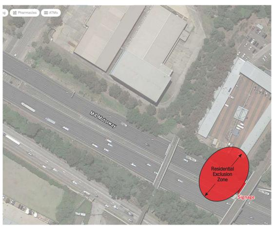
"Residential Exclusion Zone" is defined as the region in which the illuminance levels to residential properties would exceed the maximum allowable under the Zone limits in AS4282. If no residential properties are located within the Exclusion Zone then the signage will comply with the illuminance limits in the Standard.
